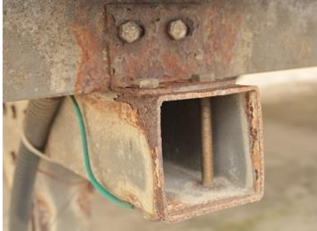
The real case in Changbin Industrial area in Taiwan. The mounting serious corrosion just after four years.
