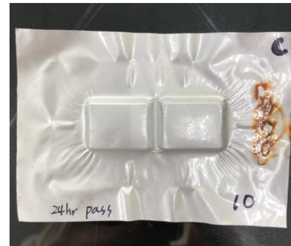
Deep drawing lab test of aluminum-plastic film of lithium batteries
