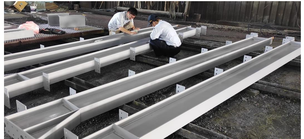
The first case in Taiwan: FEVE coating on solar cell mounting for real exposing test.
